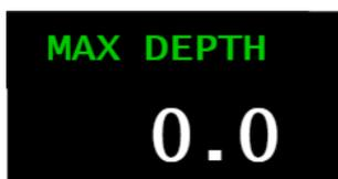
Maximum depth of the current dive in meters (displays with 1 decimal up to 999.9m) or in feet.
