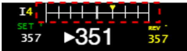
If the difference between current heading and set-point angle is over  $\pm 20^\circ$  the arrow is saturated to the left/right end of the graduated scale.
