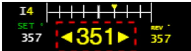
If no heading point is set then only the compass is displayed and no arrow appears.
