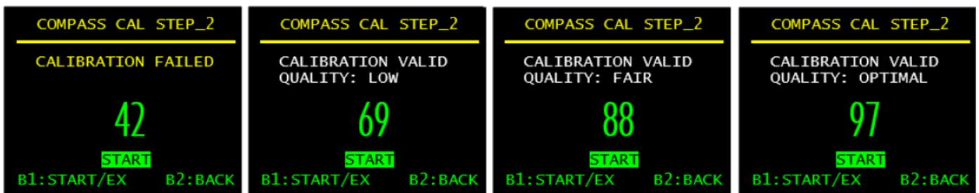
Fig 70 - STEP\_2 - Compass calibration possible results
