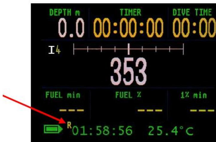
Fig 35 - Main screen - R (recording)
